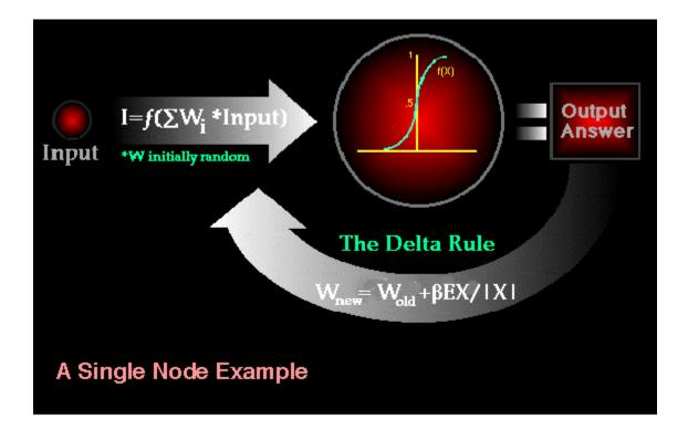
Note also, that within each hidden layer node is a sigmoidal activation function which polarizes network activity and helps it to stabilize.
