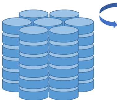
Fig. 1.13: Structure of the plastic columnar phase. The curved arrow indicates the rotational disorder of the molecules in the columns.
