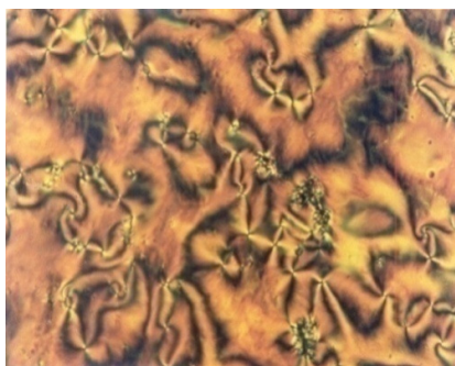
Fig. 6: Schlieren texture of SmC of 12bps at 117°C.
