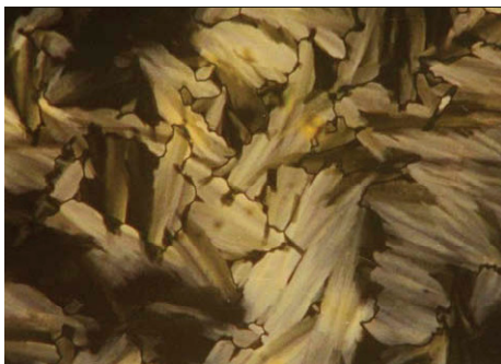
Fig. 23: POM texture of Cu-16mpd complex at 152°C (10X magnification)
