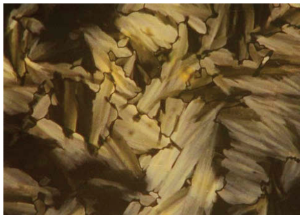
Figure 4. (colour online) POM texture of Cu-16mpd complex at 152°C (10× magnification).
