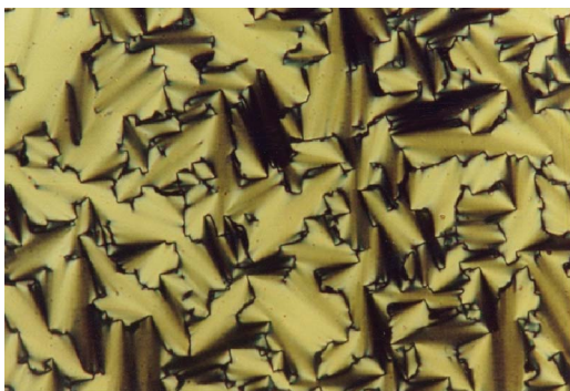
Fig. 5. Broken focal conic-shaped texture of the SmA phase at 114°C.
