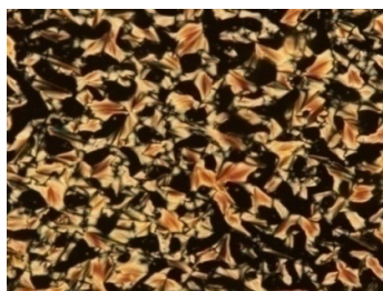
Fig.5: Broken fan-like texture of SmA phase of [\text{Dy}(\text{LH})_3(\text{NO}_3)_3] complex
