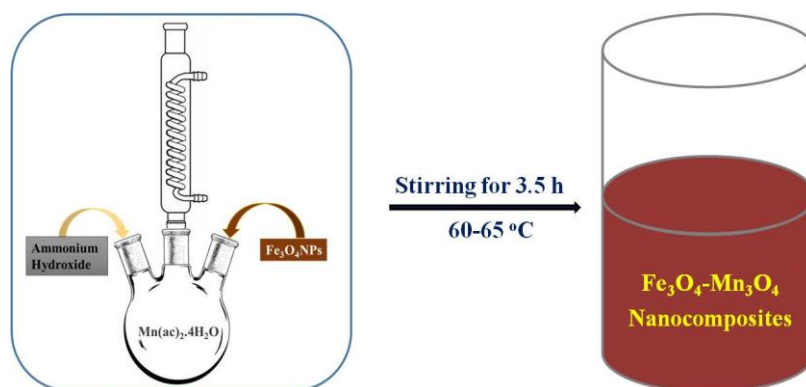
Scheme 5.1. Schematic presentation for the synthesis of Fe 3 O 4 -Mn 3 O 4 nanocomposites.
