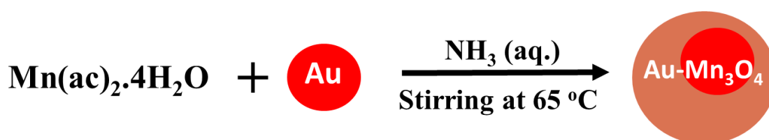
Scheme 4.1. Schematic presentation of the synthesis of Au-Mn 3 O 4 nanoparticles
