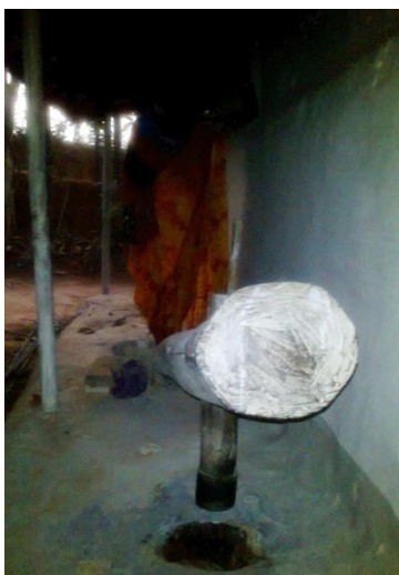
Dheki , a traditional grinding apparatus
